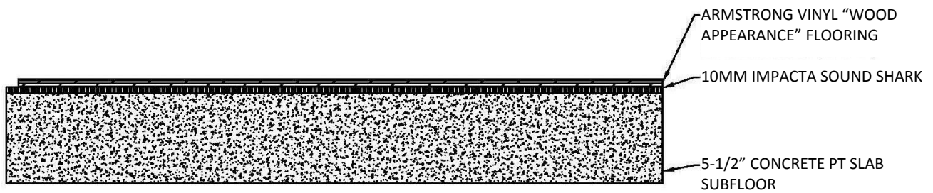
Figure 1: Floor Ceiling Assembly (Not to Scale)
